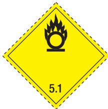
(No. 5.1) Class 5.1 Oxidizing substances Symbol (flame over circle): black; Background: yellow. Figure '5.1' in bottom corner.
