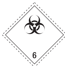
(No. 6.2) Class 6.2 Infectious substances The lower half of the label may bear the inscriptions INFECTIOUS SUBSTANCE and In case of damage or leakage immediately notify Public Health Authority. Symbol (three crescents superimposed on a circle) and inscriptions: black. Background: white. Figure '6' in bottom corner.
